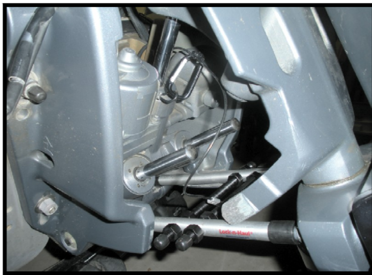
Retaining lanyard placement (Cable around hydraulic piston, and clip to cable.)
