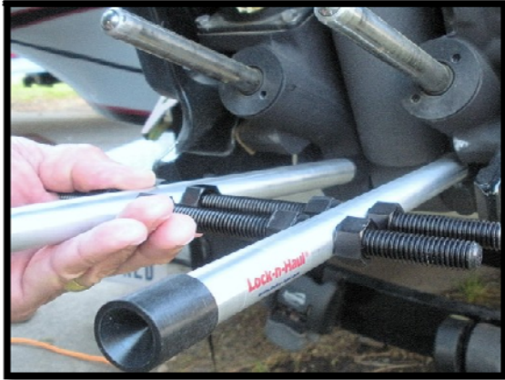
Mercury ProXS pocket placement Lower (round) tube ends near center piston
